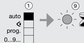
As soon as the switch is set to "auto", loading is indicated by flashing lamp "⚡". When the lamp ceases to flash, the installation is ready for operation.
