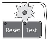
The acknowledgment LED blinks during the sending of the IR message.
