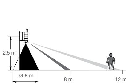
Optimal installation height is 2.5m.
