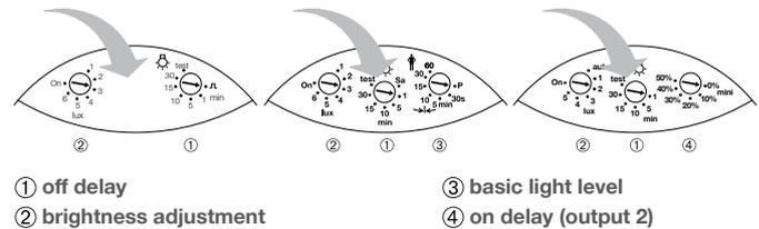
**Mode 1:** Potentiometer greater than 10° = ON delay **15 minutes**
