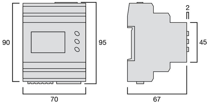
Please allow space above and below the meter for cable connections.
